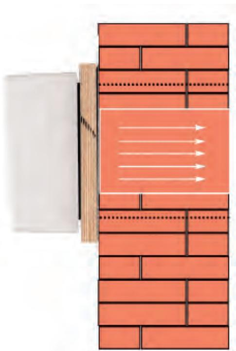
Many cellars already have core drillings, but not always with the required diameter for the fans. In order to use these core drillings also for the fans type 100-150 as well as 100-230, there is now an adapter plate available, which is mounted centrally on the existing hole.
